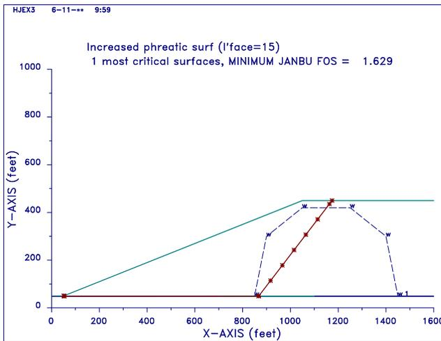
**FIGURE 5:** Engineering Slope Analysis, S.F. = 1.6.
