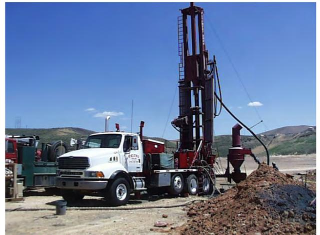
**FIGURE 7:** Dual Rotary Drill
