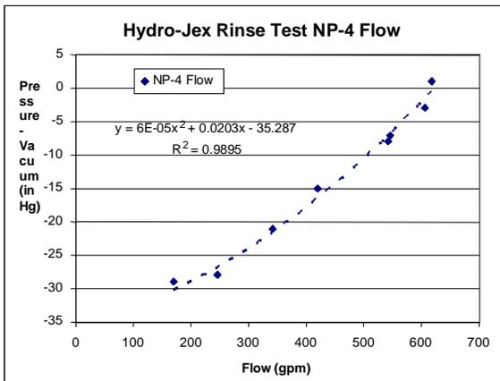
**FIGURE 15:** Wellhead vacuum (In Hg) v. Flow (gpm).
