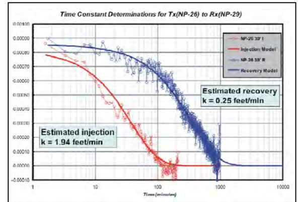
**FIGURE 12:** Hydraulic Conductivity (k) from Injection and Recovery by Geophysical Resistivity.
