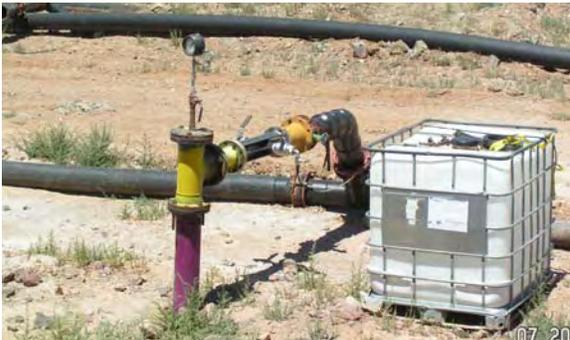
**FIGURE 14:** NaCN Solution, Air and Scale Inhibitor added to Heap via Vacuum at Wellhead.
