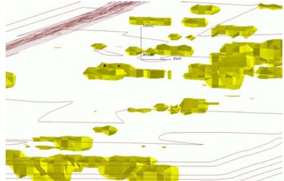
**FIGURE 5** High Resistive (Dry) Zones in a Heap Leach Pad by Geophysical Resistivity Survey.
