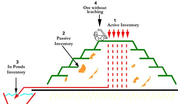
**FIGURE 3** Inventories in Heap Leaching
