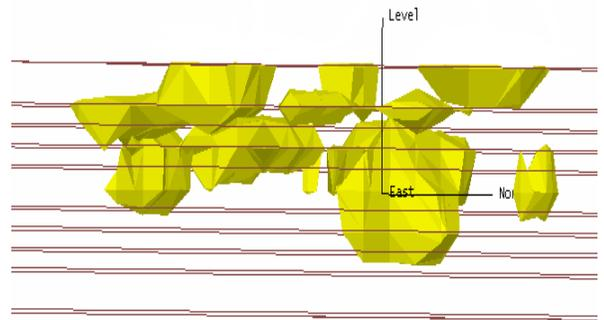
**FIGURE 6** Side View of High Resistive (Dry) Zones in a Heap Leach Pad by Geophysical Resistivity Survey.
