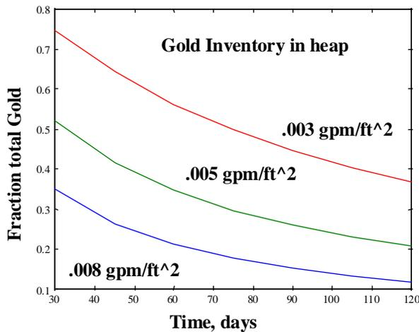
**FIGURE 8** Gold Inventory Reduction by Rinsing Application Rates.
