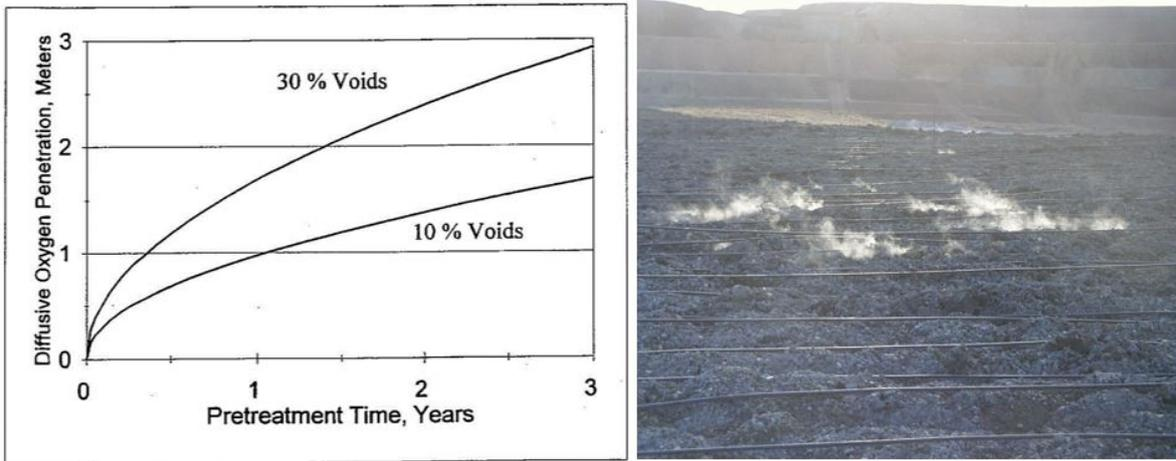
**Figures 4 and 5: Air diffusion into a heap and vapor smokes off a heap**
