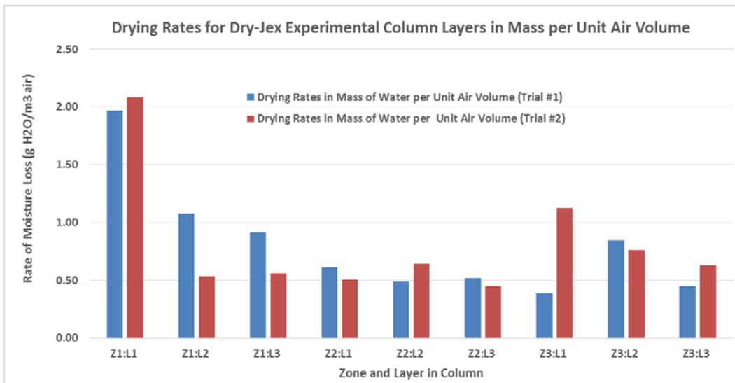
**Figure 23: Drying rates for Dry-Jex trials in mass of water loss per unit air flow (g H<sub>2</sub>O/m<sup>3</sup> air)**
