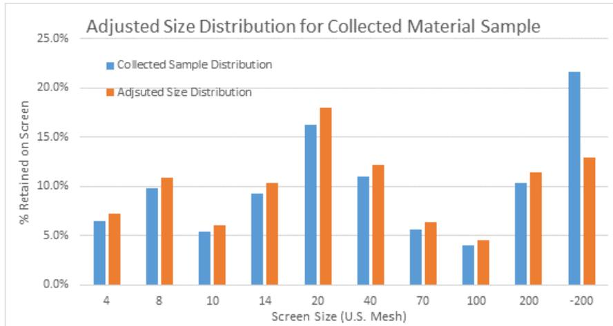
**Figure 9: Initial size distribution of material and adjustment for Dry-Jex experiment**
