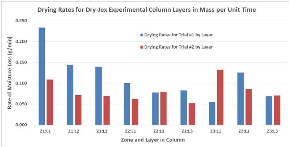
**Figure 22: Drying rates for Dry-Jex trials in mass of water loss per unit time (g/min)**
