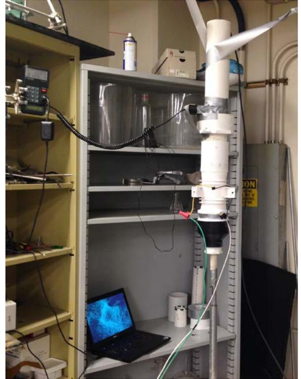
**Figures 15 and 16: Lab experiment set up: isolated barrel with material in zones with drying fan**
