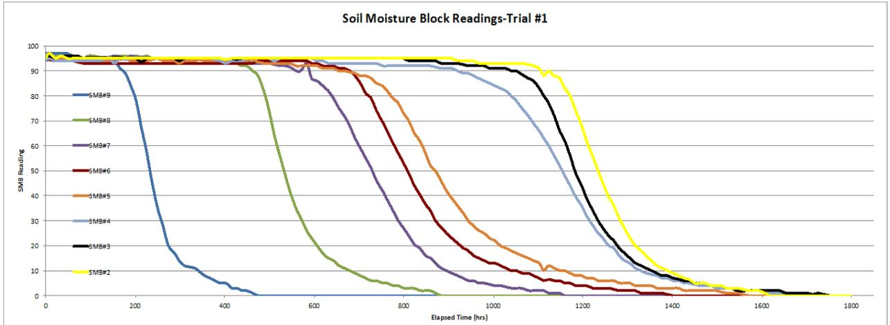
**Figure 18: SMB reading vs time for Trial #1, showing decrease in material moisture**
