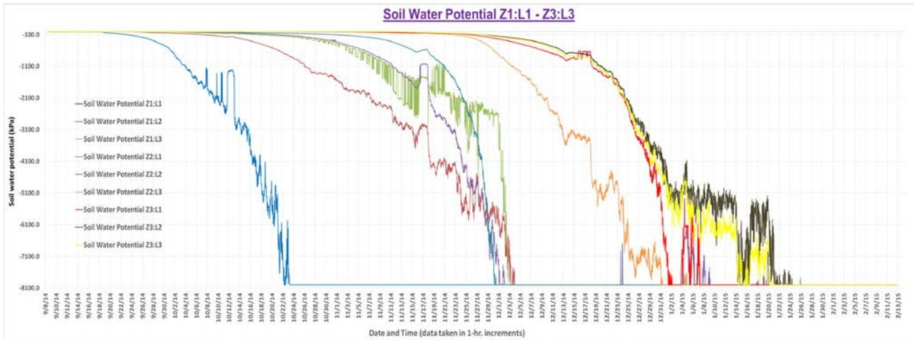
**Figure 19: Soil water potential drops versus time for Trial #2**
