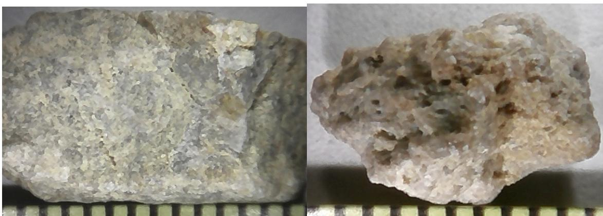
**Figures 10 and 11: +4 and +8 mesh representative particle size showing microporosity**
