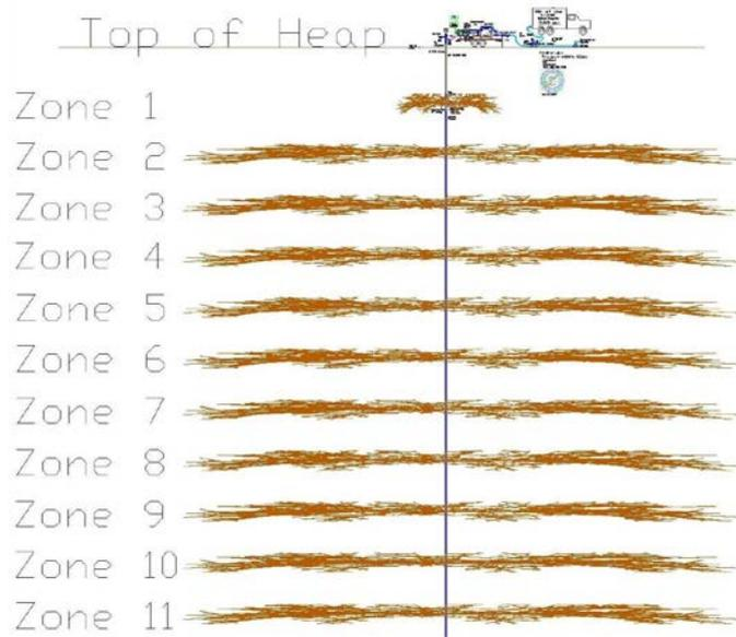
**Figure 3: Hydro-Jex zonal treatment in an ore heap**
