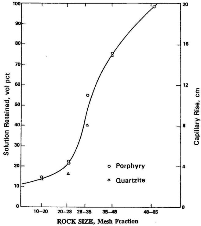
**Figure 6: Solution retention, volume % and capillary rise for various rock sizes (Tyler mesh)**
