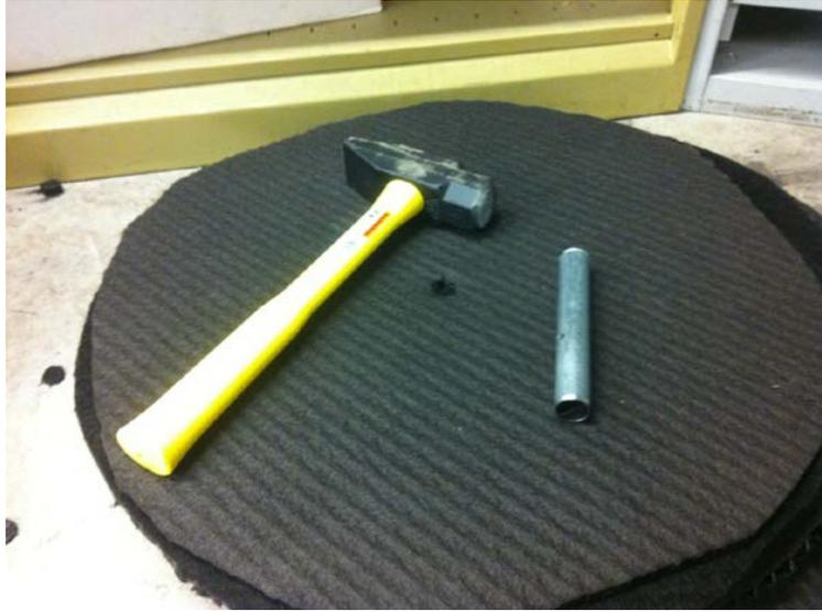
**Figure 12: Geo-composite cut to fit column**
