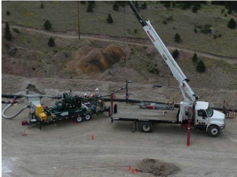
**Figure 1: Hydro-Jex solution stimulation in a heap with horizontal mixing and channelling**
