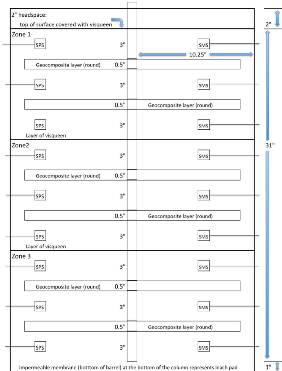
**Figure 17: Drawing of experiment showing placement of SMS-soil moisture sensors, SPS-soil water potential sensors**
